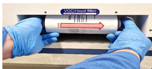
Figure 12.2 VOC/HEPA filter insertion and removal procedure
