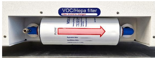
Figure 12.3 Correctly installed VOC/HEPA filter
