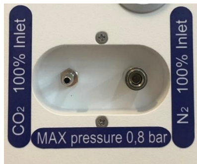
Figure 11.1 Gas inlets on the back of the MIRI® II-12 multiroom IVF incubator
